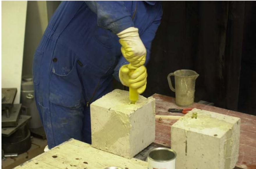
Figure 7: Grouting of cracked cubes with low pressure injector
